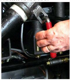
When the computer displays FILL, close the drain valve to begin refilling the frypot.
